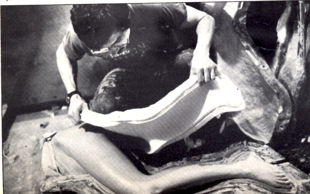
Smith's son, David, separates sections of a mold used to create full-scale, foam latex legs modeled after Catherine Deneuve's. A powerful vacuum sucked the air out of the legs, causing them to shrivel and collapse—the start of Deneuve's transformation.
